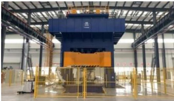
LFT-D 液压机生产线
